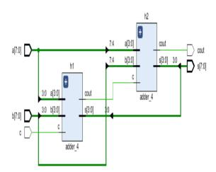
Fig.1 8 Bit Schematic Diagram
